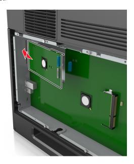
**Note:** Hold the ISP at an angle over the plastic bracket so that any overhanging connectors will pass through the ISP opening in the controller board cage.
